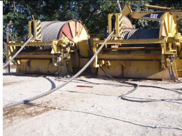
Winches Applied for Pulling Subsea Pipeline
